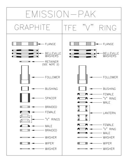
For Emission-Pak packing sets, tighten the packing nuts until the yellow line on the follower is barely visible on the top of the follower flange.
